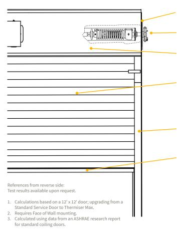
**BRACKETS** - Steel with powder coated finish to match curtain. Bolt to guide assembly and support counter-balance shaft and curtain.
